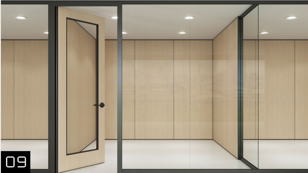
SINGLE LEAF SOLID DOOR WITH GLASS INSERT • 1-3/4” thick solid door • 6mm tempered glass insert • Soft close options • Adds visual privacy to glass storefront
