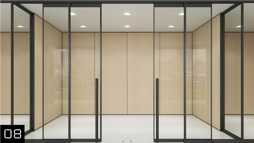
DOUBLE LEAF SLIDING DOOR • 1” thick frame, 10mm glass insert • Interior or exterior mounted rail • Standard soft close/open and bottom seal • Perfect for conference rooms and boardrooms
