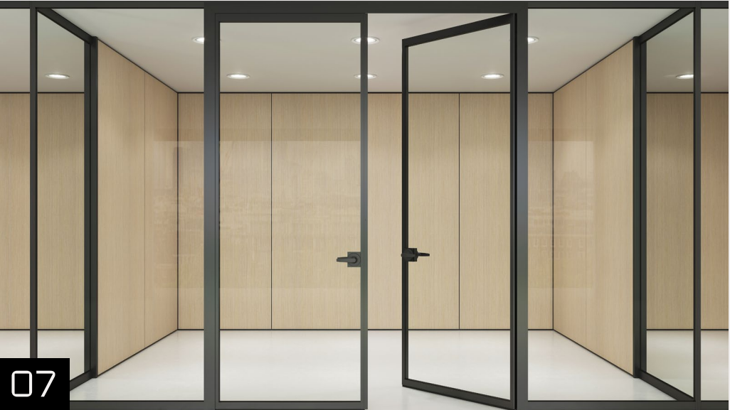
DOUBLE LEAF FRAMED DOOR • 1-3/4” thick frame, 10mm glass insert • Aluminum pivot stile • Closer and bottom seal options • Perfect for conference rooms and boardrooms
