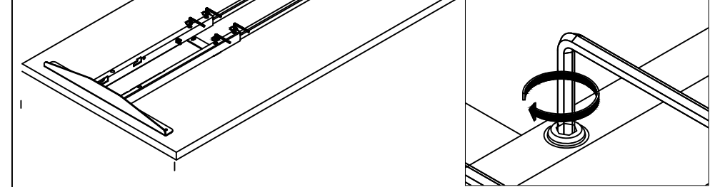
STEP 2: Attach and secure bracket to the Worksurface. Tighten the screws bracket as shown.
