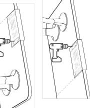
Worksurface Centerline for **BRACKET 1** Placement
