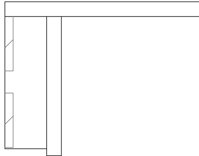
STEP 2: Simply place the Worksurface on installed Wall Cleats as shown
