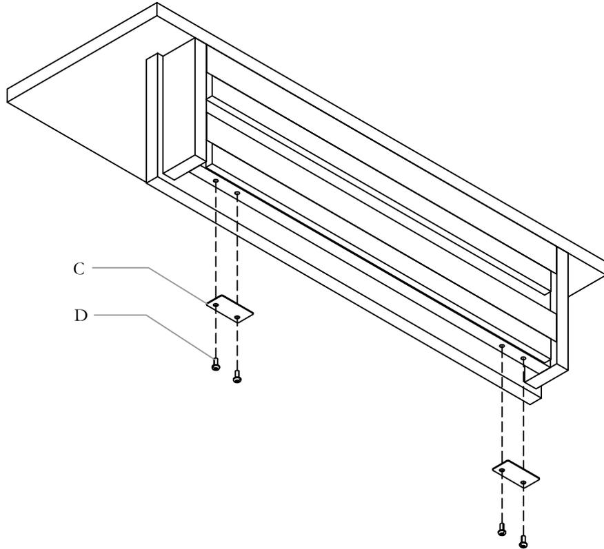
STEP 3: Install Antilift Brackets using screws as shown
