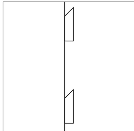
STEP 1: Install the Wood Wall Cleats as shown
