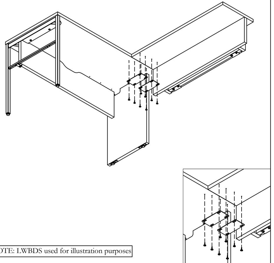
STEP 4: Tether the Worksurface with the Main Desk using Flush Plates as shown
