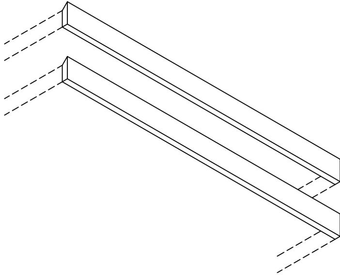
NOTE: Wood Wall Cleats will be in two splits when Surface Grommet (B) is selected for wire management purposes
