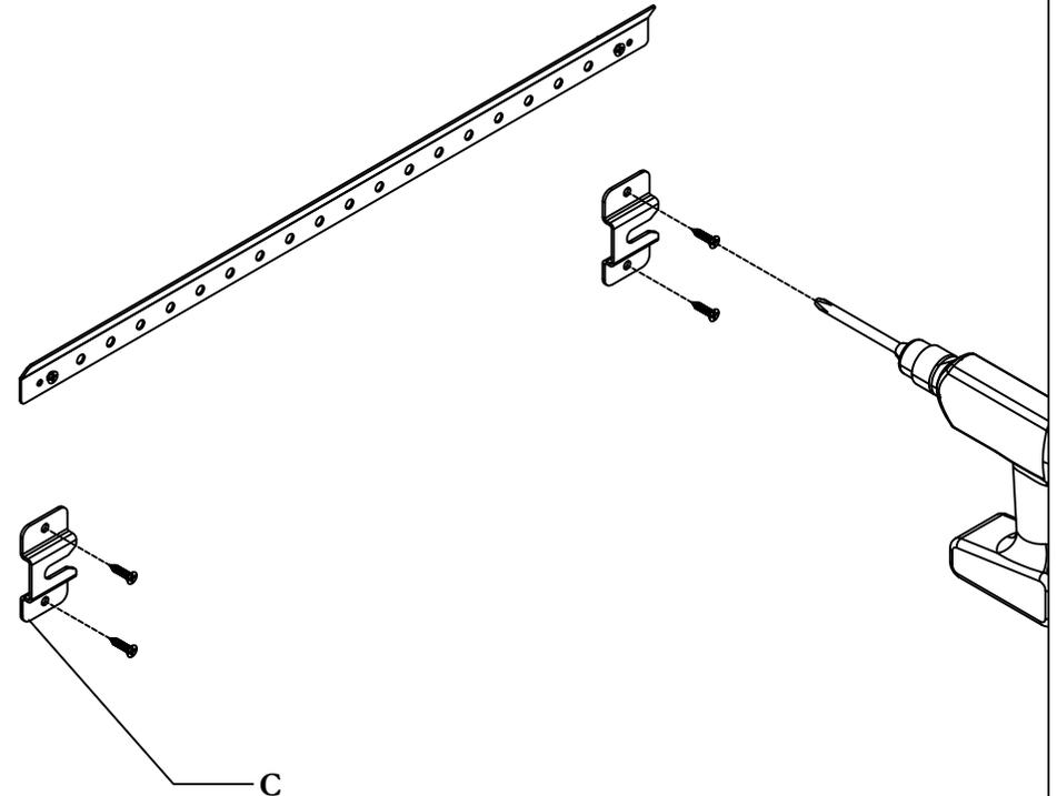
**STEP 4:** Secure the wall brackets using wall mount screws.
