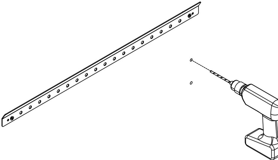
**STEP 3:** Position the wall brackets so that their edges align and they are 3.6" below the channel bracket. Mark the location of the holes and drill 2 holes for each bracket.
