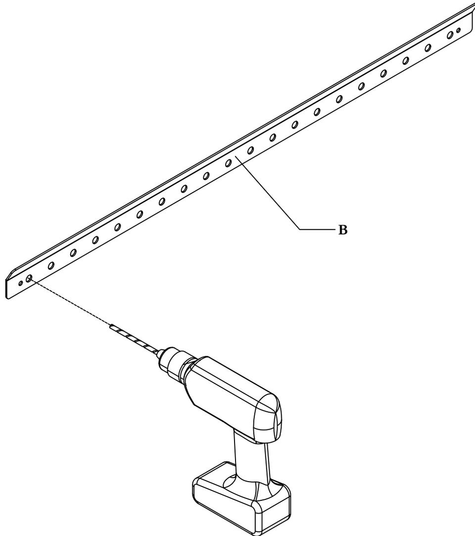
**STEP 1:** Position channel bracket on the wall. Mark the position of the holes and drill two holes in the wall.
