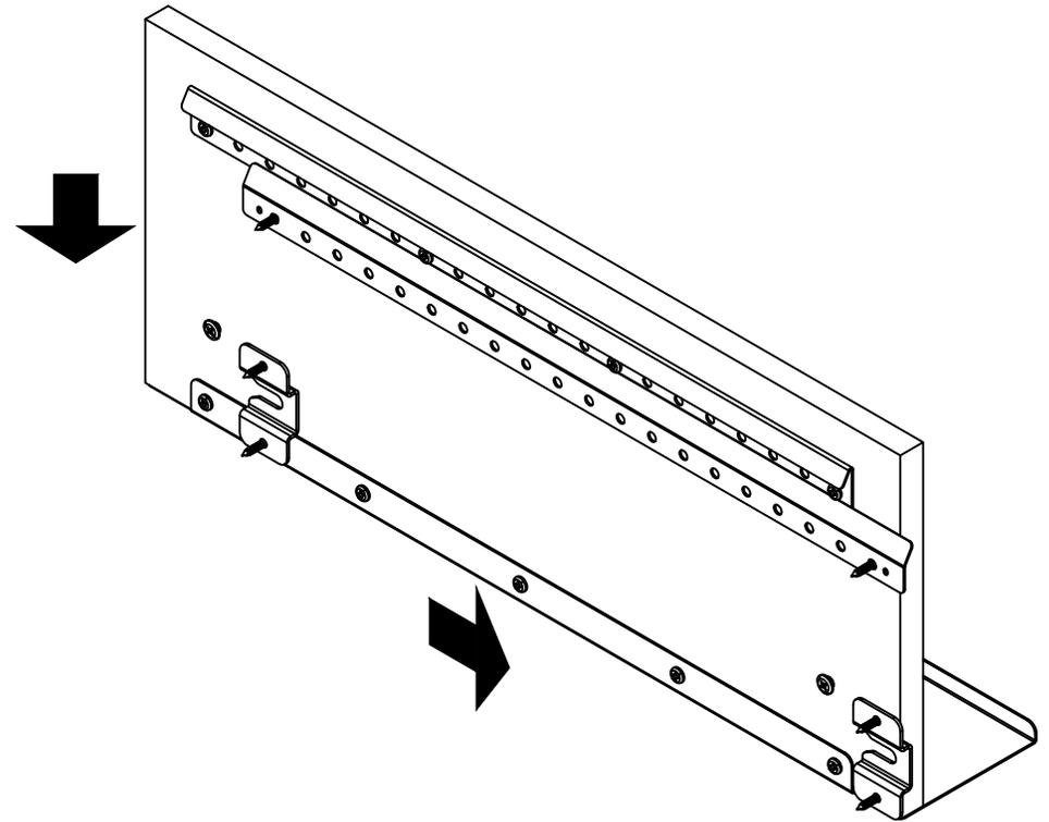
**STEP 5:** Hang the wall shelf on the wall channel bracket and slide it right to secure it with the wall brackets.
