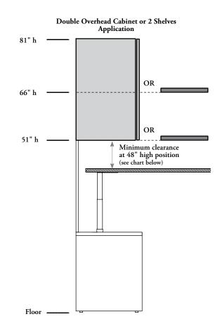
Clearance between the top of the height-adjustable worksurface and underside of the standard overhead cabinet
