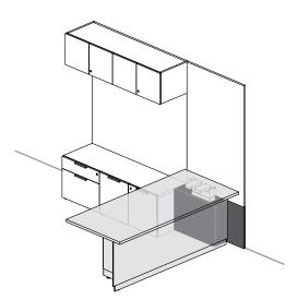
It must be specified when a wall panel is installed on a Workwall Kneespace Module for Full-Modesty. The Extension Panel **not** only offers support to the wall panel but also ensures that the worksurface depth remains completely enclosed within the wall panel
