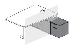
When a 46" or 52" deep Height-Adjustable Peninsula is specified above a mid-height Workwall Credenza with Open and Combo – Height-Adjustable Peninsula, the recycling/waste bins or storage section is more difficult to access, because the surface covered completely the storage access
