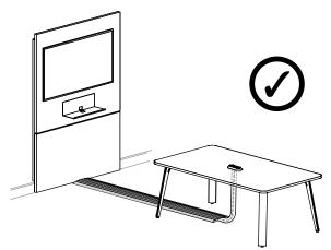
It is recommended to use the Wrap Around Cable Manager when the cables are exposed, like in the case of the cable is going straight from the cover to the worksurface
