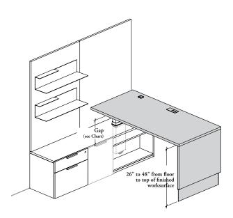
Gap between Workwall Storage for heightadjustability underneath height-adjustable worksurface
