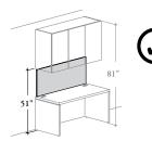
Align with bottom of Double Overhead Cabinet mounted at 81" (51)
