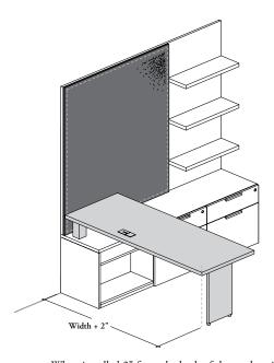
When installed 2" from the back of the workstation, the end of the worksurface is flush with front of the Tackboard or Markerboard that is mounted in front of the Wall Panel
