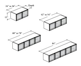
This cabinet is a lockable mounted storage unit that supplies overhead storage in a variety of widths.
