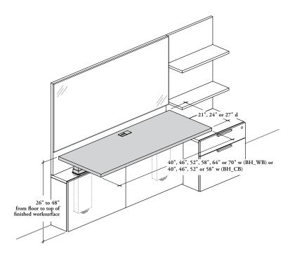
example with height-adjustable run-off (solid or glass top) & workwall credenza – height-adjustable run-off
