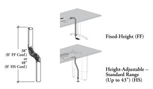
The Wrap Around Cable Manager hides and routes power and communication cables from the floor to the worksurface.
