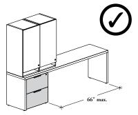
When a tower is monted on a **secondary desk** that is wider than 66", a Storage for Secondary Desk must be installed under the secondary desk to reduce its unsupported span to a maximum 66"
