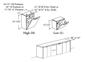
This modular service cabinet allows to provide hidden space for recycling and garbage and ensure to support secondary desk. The proper mixt of end and center storage position will allow filling the whole span of a Secondary Desk. When Yes (Y) in front of height-adjustable mechanism option is specified, the storage allows to hide the height-adjustable mechanism.
