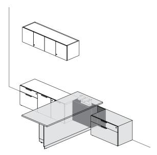
It provides a continuous aesthetic with storage on visitor side. It also preserves the mandatory 1-inch pinch gap for height-adjustable worksurface when specified with storage
