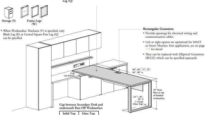
\* The recessed frame of Run-Off with Glass Top reduced the gap by 1 11/16"
