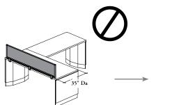
A Desk Screen **cannot** be installed on Primary Worksurface, when 35" Depth A is specified
