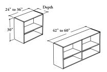
This cabinet is a mounted storage unit that supplies double overhead storage in a variety of widths.
