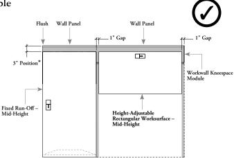
\* Three positions are available for the Fixed Run-Off – Mid-Height, when installed with Height-Adjustable Rectangular Worksurface and on kneespace module. Refer to previous page for more details
