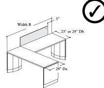
Return Worksurface: Can be specified off-module only. Use Width B minus Depth A and keep a minimum of 3" from the end of the desk
