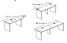
This worksurface must only be used with a Reception Desk - Straight Module (B\_CRF). It would be unstable if used alone.
