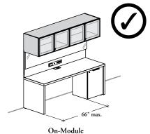
Can be installed on-module above low or high secondary desks
