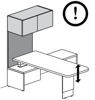
Teknion does **not** recommend the use of any overhead above the Height-Adjustable Worksurfaces. Damages or personal injuries may occur if accessories are positioned beneath the overhead
