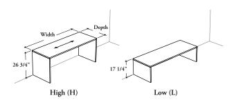
This desk provides a secondary working area (High only) and can support a fixed-height run-off worksurface (B\_MHH, BGMTH, B\_MPL, BGMTL or B\_MPG), an overlapping bridge a Wall Panel and Mounted Towers. It must be installed against a wall.
