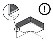
Two Desk Screens cannot be installed on module in a 90° configuration
