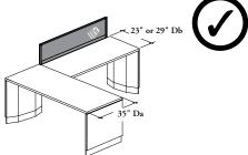
The Desk Screen can only be installed on Return when 35" Depth A is specified
