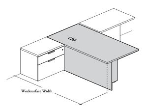
The end of the worksurface is aligned with the back of a storage and with back of the Workwall Kneespace Module
