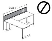
The screen on Return **cannot** be specified the same dimension than the Width B
