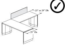
The Worksurface Edge Screen can only be installed on Return when 35" Depth A is specified
