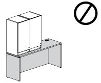
Towers **cannot** be mounted on a **standard desk**. They can only be supported by a Low or High Secondary Desk
