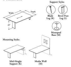
This 29" fixed-height meeting peninsula must only be mounted on a Workwall Srorage (BHKHF, BHKFW, BSMOBW) or a Media Wall (BCMW). Perfect for virtual meetings and presentations. The table offers both power and data access for laptops, as well as seamless connectivity to the screen.
