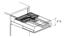
• 4" high standard box drawer allows to stack its Pencil Tray over the Box Drawer Organizer. Both items must be placed side-by-side in a 3" high small box drawer
