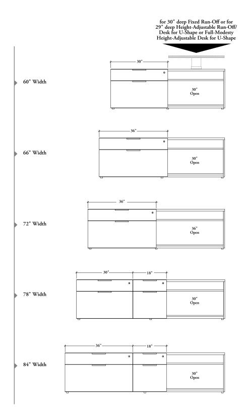
workwall credenza with with open & drawers – fixed worksurface mid – 21" h (BSMWL) or workwall credenza with with open & drawers – height-adjustable run-off – mid – 21" h (BSMHLR) workwall credenza with with open & drawers – height-adjustable peninsula – mid – 21" h (BSMHDP)
