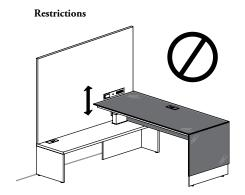
The Power Bar and Cover on Wall Panel cannot be specified over height-adjustable worksurface, as it may lead to conflicts with plugged-in power
