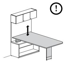
Teknion does not recommend the use of any overhead cabinet or shelves above the Height-Adjustable Worksurfaces. Damages or personal injuries may occur if accessories are positioned beneath the cabinet. The use of a TV Stand is impossible in this application.
