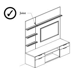
Example of joint position with a smaller shelf (24" and 60" widths) specified
