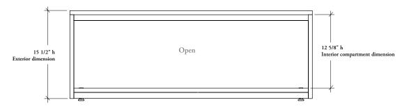
Bookcase – Secondary Desk – Center or End Position – Low Secondary Desk For end position storage, the interior compartment dimension is the same for 1 3/16" (M) or 1 9/16" (X) worksurface thickness
