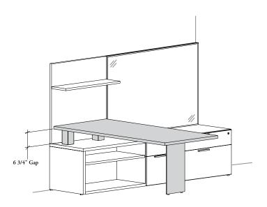
Worksurface thickness does not affect clearance gap
