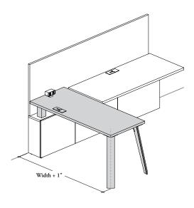
When installed 1" from the back of the workstation, the end of the worksurface is flush with front of the Wall
