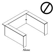
Cannot be used alone. It must always be connected to a Main Worksurface or standard desks for stability
