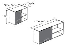
This cabinet is a lockable mounted storage unit that supplies double overhead storage in a variety of widths.
