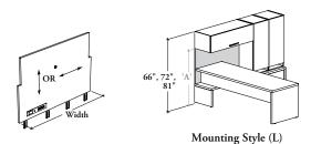
This wall panel is designed to support an overhead cabinet. It is compatible with tackboard or markerboard for enhanced functionality. Whether mounted onto a desk, credenza, secondary desk, mid-height storage, workwall kneespace module or workwall credenza, the wall panel is easily installed requiring securement at only two wall locations.
