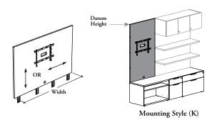
This wall panel supports the integration of technology and TV monitor in the office. Whether mounted onto a desk, credenza, secondary desk, mid-height storage, workwall kneespace module or workwall credenza, the wall panel is easily installed requiring securement at only two wall locations.
