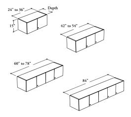
This cabinet is a lockable mounted storage unit that supplies overhead storage in a variety of widths.
