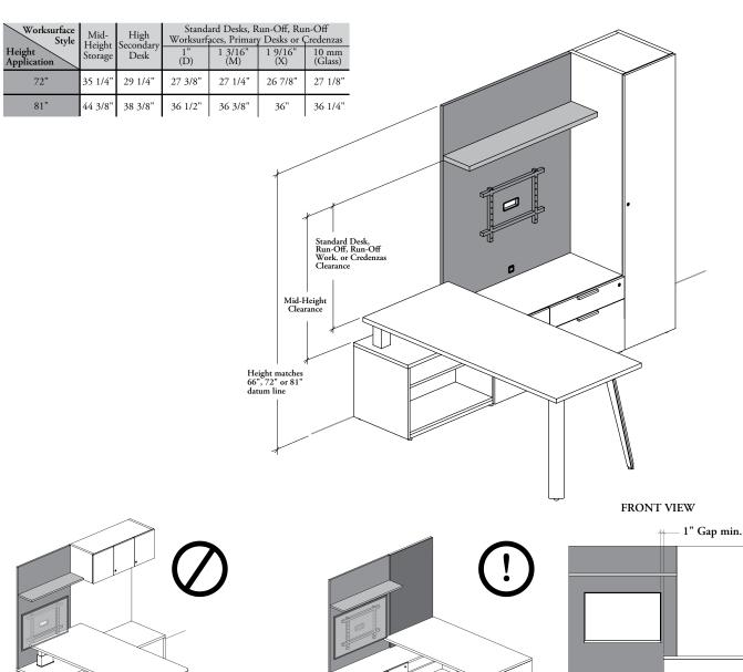
Wall Panel for Media and shelf **cannot** be specified over a height-adjustable worksurface
