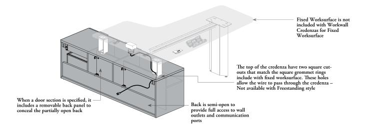
components & cable routing on standard or height-adjustable worksurface supporting style
