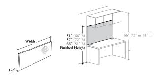
This fabric-wrapped tackboard is a low-cost alternative and it installs under any Wall-Mounted Overhead Cabinet.
