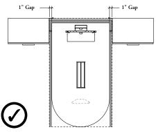
$\begin{array}{l} \mbox{Minimum clearance between Height-Adjustable} \\ \mbox{Meeting Peninsula } (B\_HRW, B\_HDW \mbox{ and} \\ \mbox{B\_HBW)} \mbox{ and a storage} \end{array}$
