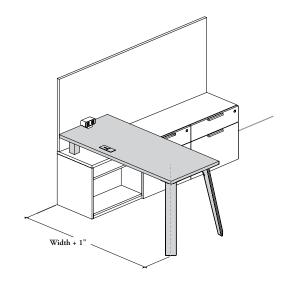
When installed 1" from the back of the workstation, the end of the worksurface is flush with front of the Wall Panel
