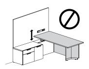
A Power Bar and Cover included with Wall Panel cannot be aligned with the end of a Full-Modesty Height-Adjustable Worksurface because the worksurface interfered with electric plugs. Refer to page 266 for details
