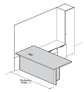
When installed 1" from the back of the workstation, it allows to install the worksurface flush with the front of the Wall Panel
