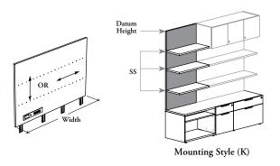
This wall panel bring a distinctive architectural element to the office desk. It is designed to support soild shelves and is compatible with tackboard or markerboard for enhanced functionality. Whether mounted onto a desk, credenza, secondary desk, mid-height storage, workwall kneespace module or workwall credenza, the wall panel is easily installed requiring securement at only two wall locations.
