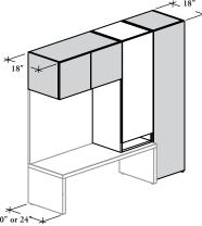
All 18" depth available in Standard Overhead Cabinets –Wall Panel Mounted (BOSHW, BOGHW, BOSSW, BOGSW, BOSOSW, BOSOGW or BOCOLW), Double Overhead Cabinets –Wall Panel Mounted (BODSHW, BODGHW, BODSSW or BODGSW), Mounted Towers and freestanding Towers can achieve a flush front look
