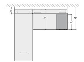
When positioned in front a Workwall Kneespace Module, drawer fronts of 20" depth storage is designed to align with 27" depth height-adjustable worksurface
