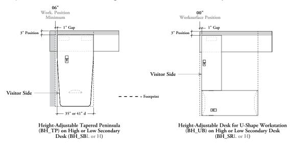
Solid height-adjustable worksurfaces for 46" deep Height-Adjustable Extended Tapered Peninsula or all styles L-Shape Worksurfaces allows a 1" gap on visitor and user sides
