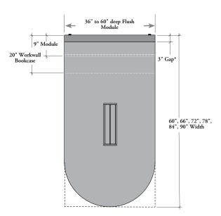
When used with a Fixed Meeting Peninsula (BC\_FR, BC\_FS or BC\_FT) and a mid-height suppport, the worksurface will be flush with the sides of the Workwall Storage
