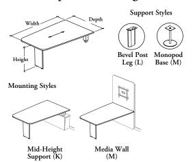
This fixed-height meeting peninsula must only be mounted on a Workwall Srorage (BHKHF, BHKFW or BSMOBW) or a Media Wall (BCMW). Perfect for virtual meetings and presentations. The table offers both power and data access for laptops, as well as seamless connectivity to the screen.
