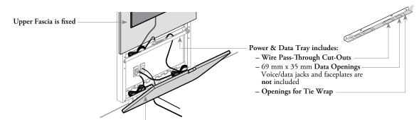
Bottom Fascia can be removed to allow access and maintenance to building power and communication outlets, while adding aesthetic
