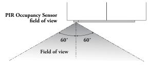
When a temperature change is detected in the field of view, the PIR shut-off timer resets to 20 minutes
