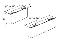
This module supports a Height-Adjustable Worksurface to enable users to work facing the wall in a sit/stand position. It must be anchored to a building wall.
