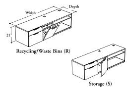
This credenza supports Fixed Worksurface while providing convenient storage areas with shelving, door section with optional recycling/waste bins and filing.
