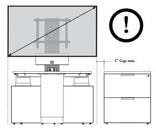
When the TV Monitor width exceeds the surface width, always keep a 1" gap with surrounding object or furniture to avoid collision hazard.
