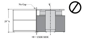
**WARNING:** When used with Height-Adjustable Peninsula (BH\_RP) or Height-Adjustable Tapered Peninsula (BH\_TP), surrounding storage on user side **MUST BE** specified Mid-Height Datum (21" height) to avoid conflict with worksurface. If **not**, 1" pinch gap must be preserved
