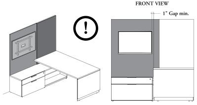
A minimum of 1" gap must be preserve between the monitor mounted on the wall panel and the adjacent height-adjustable worksurface to avoid potential damage or injury
