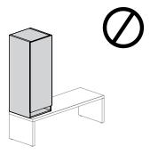
A mounted tower **cannot** be installed alone on a secondary desk. It must be connected with another product for more stability. See the illustrations below for the multiple possibilities
