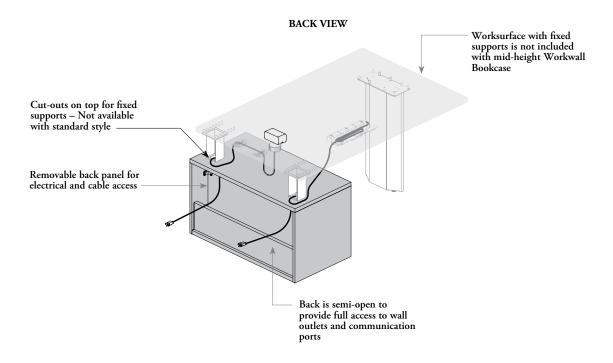
components & cable routing for height-adjustable configurations (standard or supporting (shown) style)
