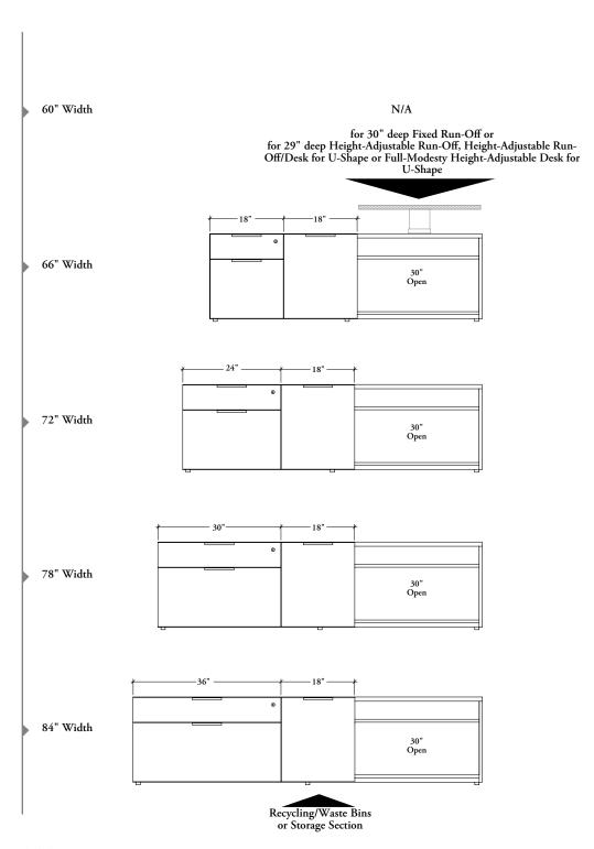
workwall credenza with with open & combo – fixed-worksurface – mid – 21" h (BSMCFW) or workwall credenza with with open & combo – height-adjustable run-off – mid – 21" h (BSMCHR) workwall credenza with with open & combo – height-adjustable peninsula – mid – 21" h (BSMHCP)
