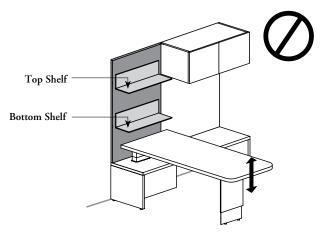
The bottom shelf on Wall Panel cannot be specified over a height-adjustable
