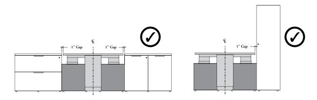
When the Workwall Kneespace Module or Bookcase is used with a Height-Adjustable Meeting Peninsula (B\_HRW, B\_HDW or B\_HBW) the combination of products will automatically ensure the 1" minimum clearance all around worksurface
