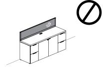
Cannot be installed on credenza with no open section (B\_ZFL, B\_ZFS, B\_ZFD, B\_ZFDB, B\_ZFDF)
