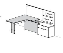
Workwall Kneespace Module – Height-Adjustabilty combined with Height-Adjustable L-Shape Tapered Peninsula
