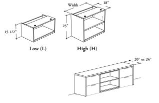
This modular bookcase allows to provide additional storage and ensure to support secondary desk. The proper mixt of end and center storage position will allow filling the whole span of a Secondary Desk. When Yes (Y) in front of height-adjustable mechanism option is specified, the storage allows to hide the mechanism.
