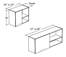
This cabinet is a mounted storage unit that supplies double overhead storage in a variety of widths.
