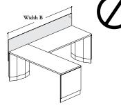
A screen on Return cannot be specified the same dimension than the Width B
