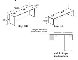
This desk supports a Height-Adjustable L-Shape Worksurfaces (BH\_LB, BH\_L, BH\_LT), a Wall Panel and Mounted Towers. It must be installed against a wall.
