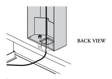
The Back Cover can be opened to route cables through the Square Grommet
