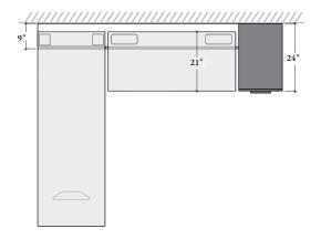
When positioned beside a Workwall Kneespace Module, drawer fronts of 24" depth storage is designed to align with 21" depth height-adjustable worksurface
