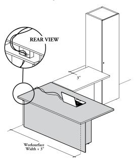
When installed 3" from the back of the module, it allows alignment with adjacent height-adjustable worksurface. A gap is created to manage wires and reach the mid-height module through worksurface support
