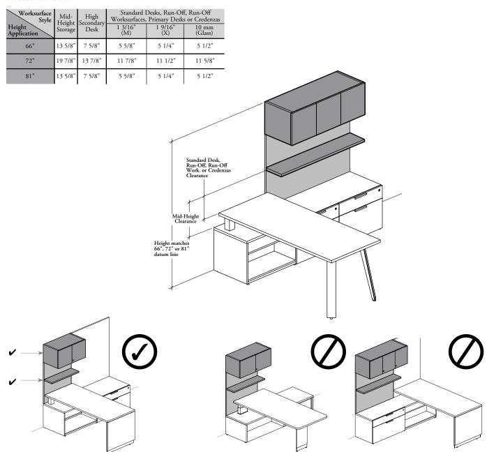
Overhead Cabinet and Shelf on Wall Panel (B\_WCO) can be used over the fixed worksurface on the Workwall Credenza without conflict
