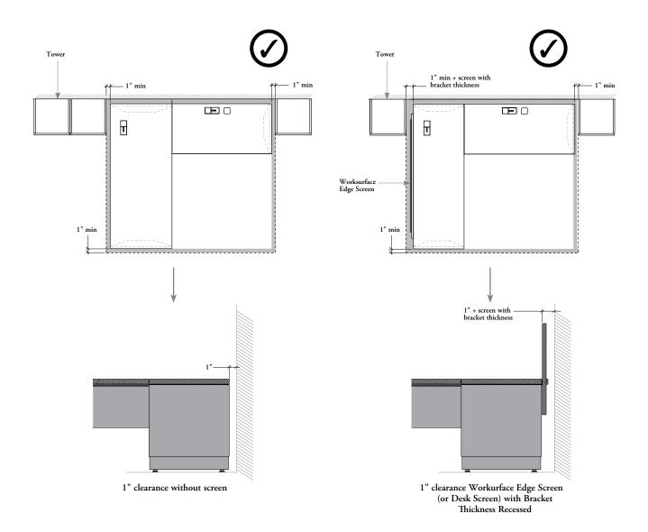
With Worksurface Edge or Desk Screen a minimum 1" clearance must be maintained
