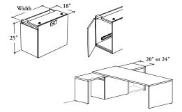
This modular storage allows to provide additional storage and ensure to support secondary desk. It can be used in conjunction with other storage for secondary desk in order to fill the whole span of a secondary desk. When Yes (Y) in front of height-adjustable mechanism option is specified, the storage allows to hide the heightadjustable mechanism.
