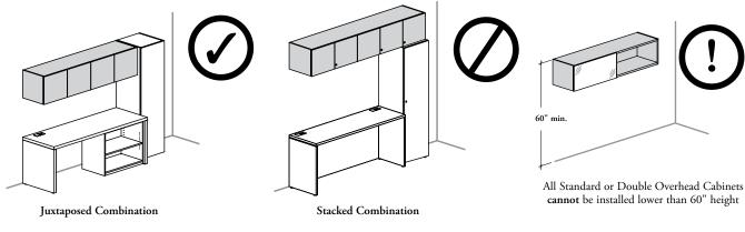
A tower or storage can be installed beside a wallmounted overhead cabinet
