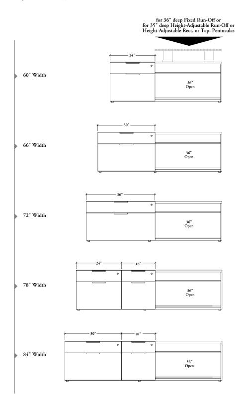
workwall credenza with with open & combo – fixed-worksurface – mid – 21" h (BSMCFW) or workwall credenza with with open & combo – height-adjustable run-off – mid – 21" h (BSMCHR)
