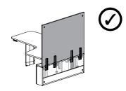
A Wall Panel mounts onto the rear side of a Workwall Kneespace Module
