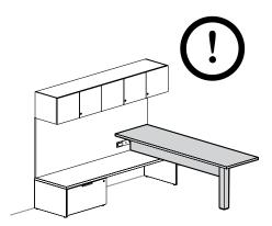
Position of modesty panel can interfere with under-worksurface power and data specified on the Wall Panel. Use specification software appropriately
