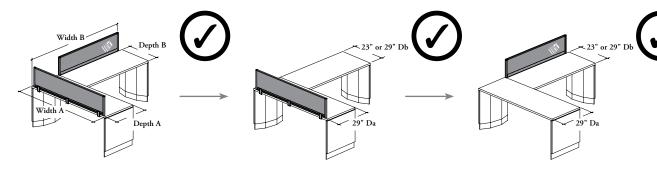
Can be installed on primary and return worksurfaces at the same time
