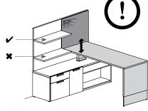
The bottom solid shelf cannot be specified right next to a height-adjustable worksurface because it may interfere. This interference only occur when specifying a Height-Adjustable Run-Off with Bevel Base (BH\_RB or BHGRB) and Height-Adjustable Peninsula with Bevel Post Leg (BH\_RP or BH\_TP)
