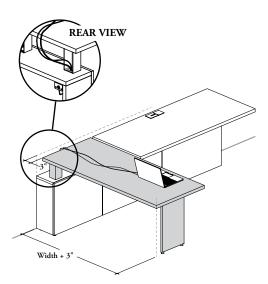
When installed 3" from the back of the module, it allows alignment with adjacent height-adjustable worksurface. A gap is created to manage wires and reach the mid-height module through worksurface support
