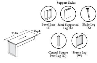
This worksurface must only be mounted on a Low Secondary Desk (B\_MSD) and attached to a wall panel at one end and is supported by a single support at the other.
