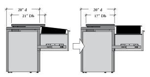
It is not recommended to specify the return of a L-Shape Worksurface deeper than the Secondary Desk, when in combination with a Lateral File – Secondary Desk (BSSL)
