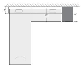
When positioned beside a Workwall Kneespace Module, drawer fronts of 20" depth storage is designed to align with 17" depth height-adjustable worksurface
