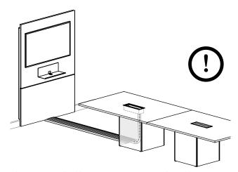
The Wrap Around Cable Manager is **not** necessary when cables are completely out of range from the user, like when the cables pass through a table base
