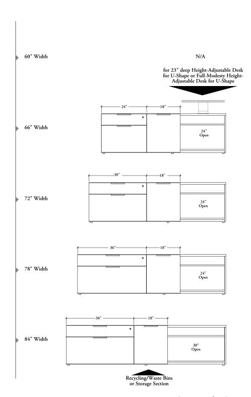
workwall credenza with with open & drawers – fixed worksurface – mid – 21" h (BSMWL) or workwall credenza with with open & drawers – height-adjustable run-off– mid – 21" h (BSMHLR)
