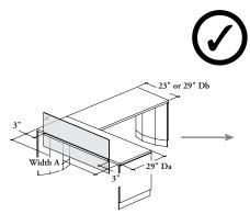
Primary Worksurface: Can be specified offmodule only. To determine the width of the screen, a minimum of 3" gap must be kept on each side of the desk
