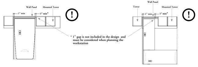
Minimum clearance allowed between Height-Adjustable Tapered Peninsula, a Mounted Tower on both sides and a Wall Panel
