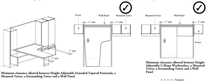
Special considerations must be taken when planning these following combinations of products, since the 1" minimum clearance required all around the height-adjustable worksurface will not be automatically ensured
