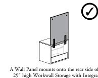
A Wall Panel mounts onto the rear side of a 29" high Workwall Storage with Integral Top
