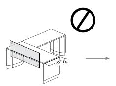
Worksurface Edge Screen cannot be installed on Primary Worksurface, when 35" Depth A is specified
