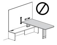
A Power Bar and Cover included with Wall Panel cannot be aligned with the end of a Height-Adjustable Worksurface because the worksurface interfered with electric plugs. Refer to page 266 for details
