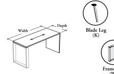
This desk must only be used in conjunction with the Overlapping Bridge (B\_MBH or B\_MBL) or Overlapping Bridge with End Support (B\_MBG) to create a "U" configuration. It would be unstable if used alone.
