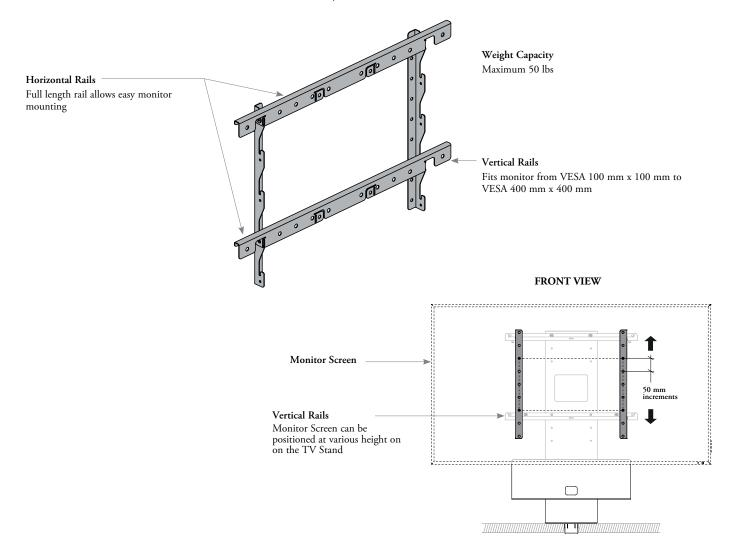
Come with fixation holes to lock the monitor in place and to ensure the monitor is centered on the tile
