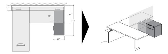
When a 42" wide Mid-Height Credenza is specified perpendicular to a 27" deep worksurface, a small portion of the drawers will be under the worksurface
