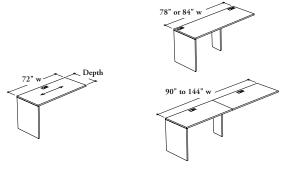
This worksurface must only be used in conjunction with a Reception Desk – L-Shaped Module (B\_CRL) to create a "L" configuration. It would be unstable if used alone.
