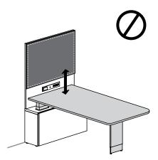
• A Power Bar and Cover included with Wall Panel cannot be aligned with the end of a Height-Adjustable Meeting Peninsula because the worksurface would interfere with electric plugs. Refer
