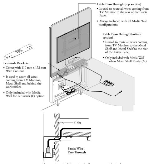
1" gap at the end of the peninsula allows to route cables in the bracket opening and reach the back of the Media Wall through a fascia space gap
