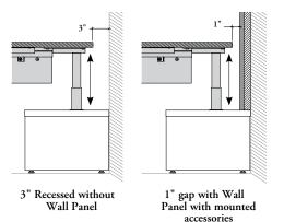
Minimum clearance allowed between Height-Adjustable U-Shape Desk, a Mounted Tower, a freestanding Tower and a Wall Panel
