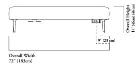
Banqs is available with electrical modules mounted below the seat. The centerline of the module is always 9" (23 cm) from the outside edge of the bench and can be specified left or right.
