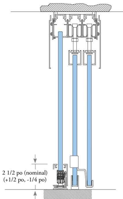
Rail de plancher Telescope (FQFB)
