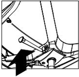
Seat height can be adjusted by lifting the lever underneath the seat on the right side. When the lever is lifted up, the weight of the body will cause the seat to lower. Releasing the lever stops the seat at the desired height. Lifting the lever up with no weight on the seat allows it to rise.
