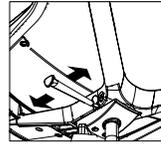
Moving the lever found under the right side of the seat locks and unlocks the recline. Push lever forward to lock chair in upright position. Pull the lever backwards to unlock for tilting action.
