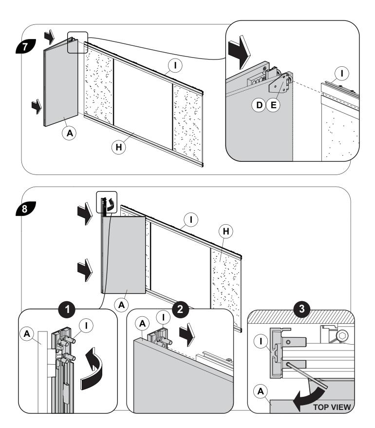
I **D**(**E**) A Α NOTE: Η Repeat steps 7 and 8.  $\square$ DOOR HEIGHT ADJUSTMENT **FRONT VIEW** 10 **UPWARD ADJUSTMENT** DOWNWARD ADJUSTMENT Ε L L D 0 0 A 0 0 A 0 0 0  $(\mathbf{D})$ WARNING: To avoid damage, adjust E top and bottom hinges alternately.
